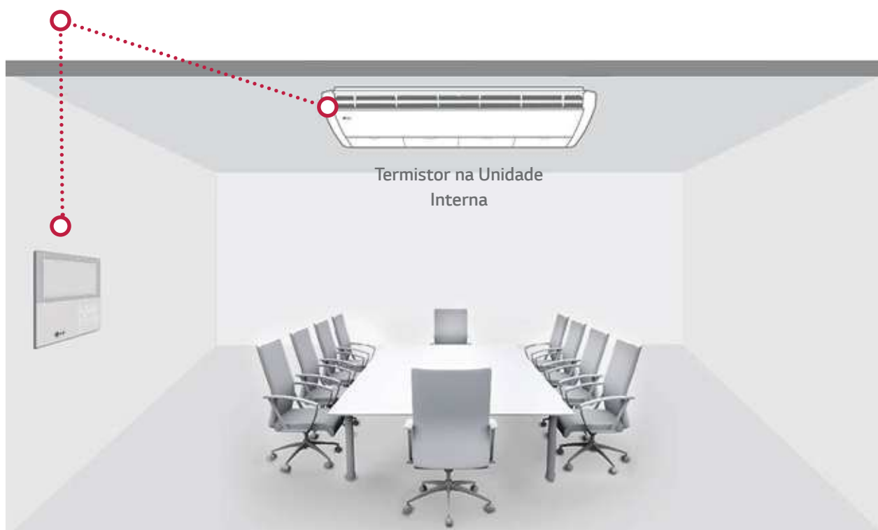
Termistor no Controle Remoto
