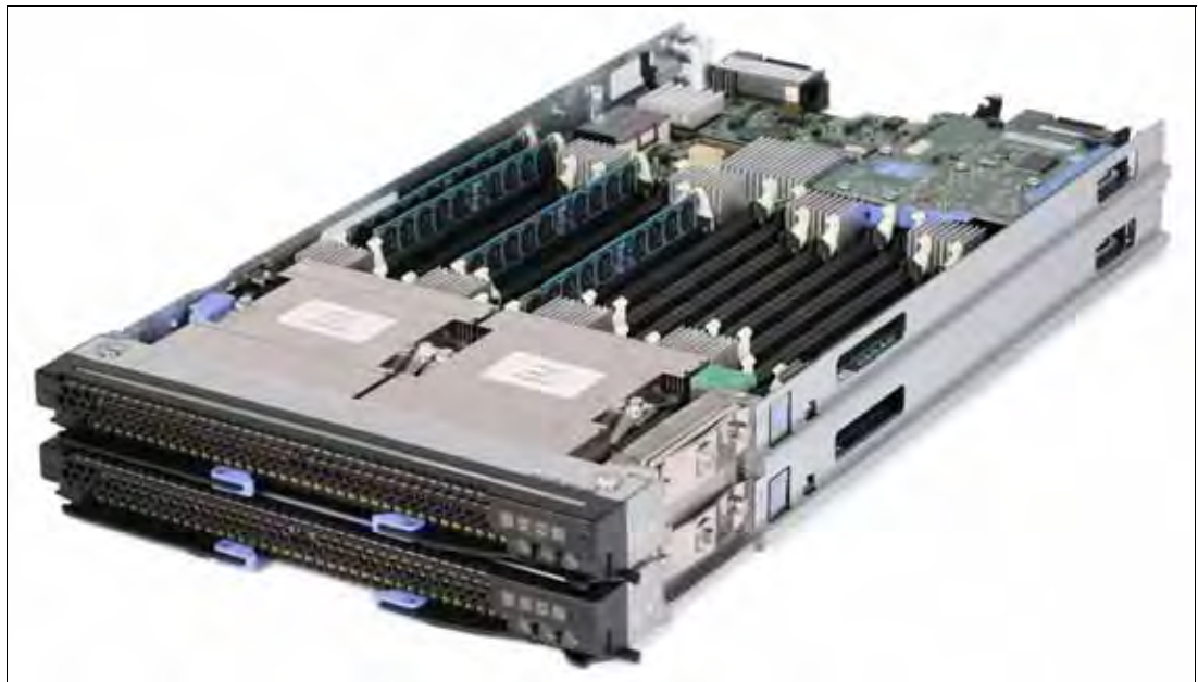
Figure 1-14 HX5 (two servers shown, connected to form one single-image four-socket server)
