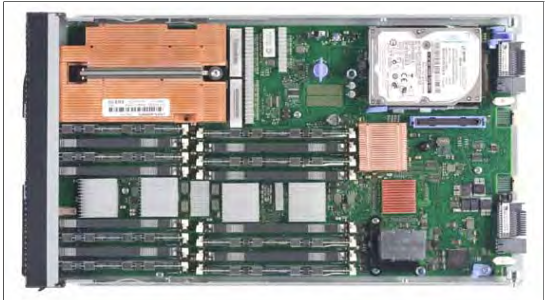
Figure 1-16 The internals of the BladeCenter PS702 blade server (showing the top half)
