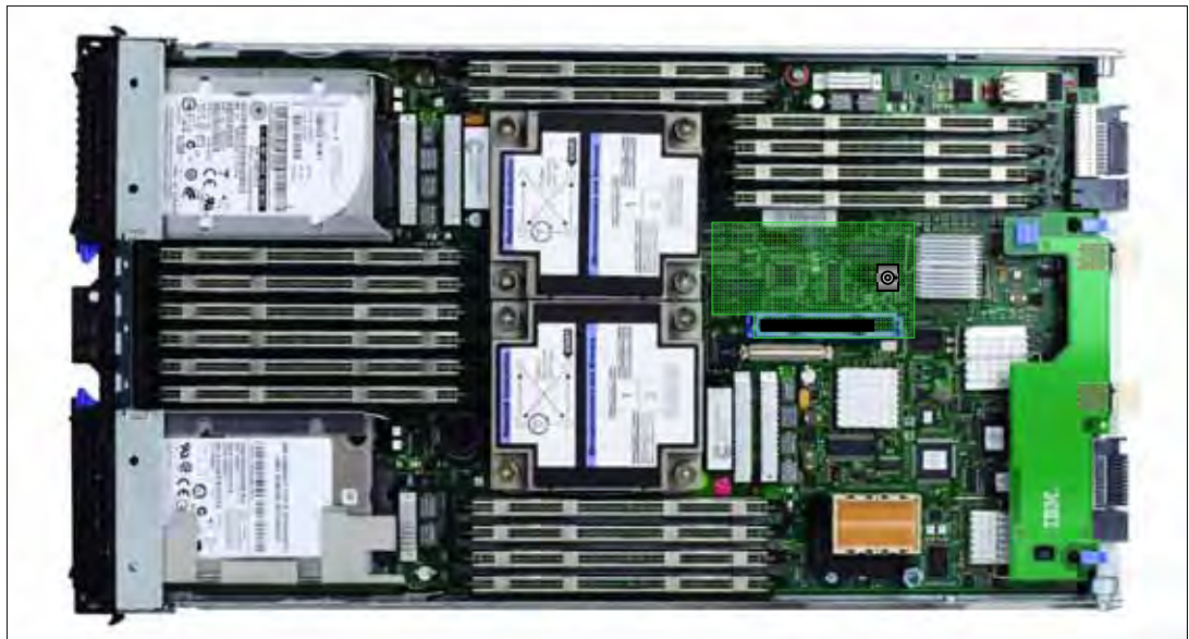
Figure 3-44 The HS23 type 7875 showing the CIOv I/O expansion card position
