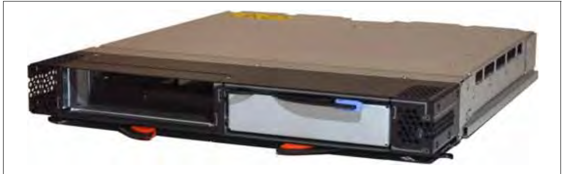
Figure 2-48 Multi-Switch Interconnect Module for BladeCenter HT (without interposers)
