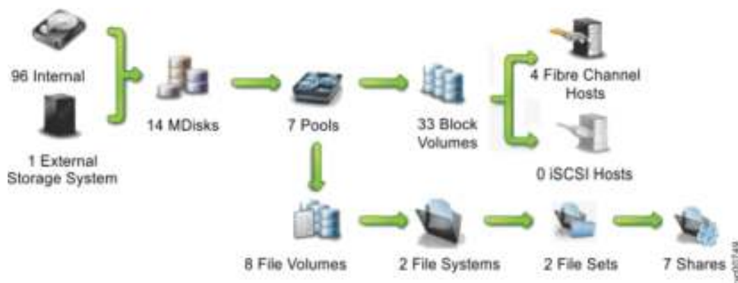
Figure 4. Storwize V7000 Unified components
