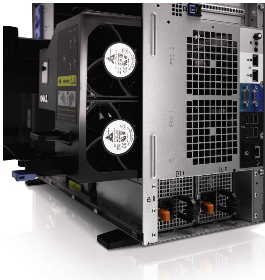
Figure 5. Fans and Cooling Shroud
