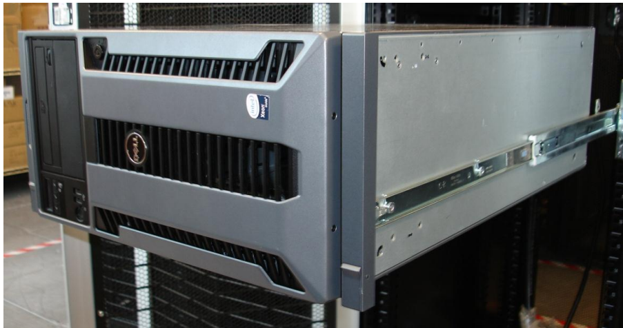
Figure 12. T610 Mounted in C1 Sliding Rails
