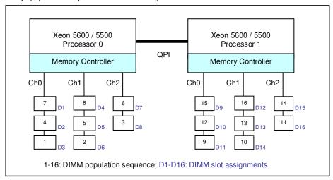
The **E5603**, **E5606**, **E5607**, and **E5620** processors support up to **1066MHz** clock speed. Using 1066MHz memory (where supported) versus 800MHz offers up to **28**% better performance. **X5650** through **X5675** processors, supporting up to 1333MHz clock speed, are available via CTO,
