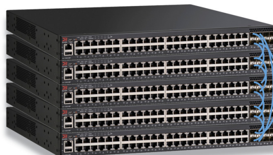
Figure 1: Up to 12 Brocade ICX 7250 Switches can be stacked together using up to four full-duplex SFP+ 10 Gbps ports for a fully redundant backplane with 80 Gbps of stacking bandwidth.
