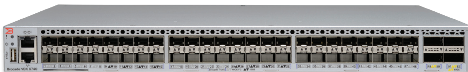
Figure 1: The Brocade VDX 6740 Switch provides 48 10 GbE SFP+ ports and four 40 GbE QSFP+ ports.
