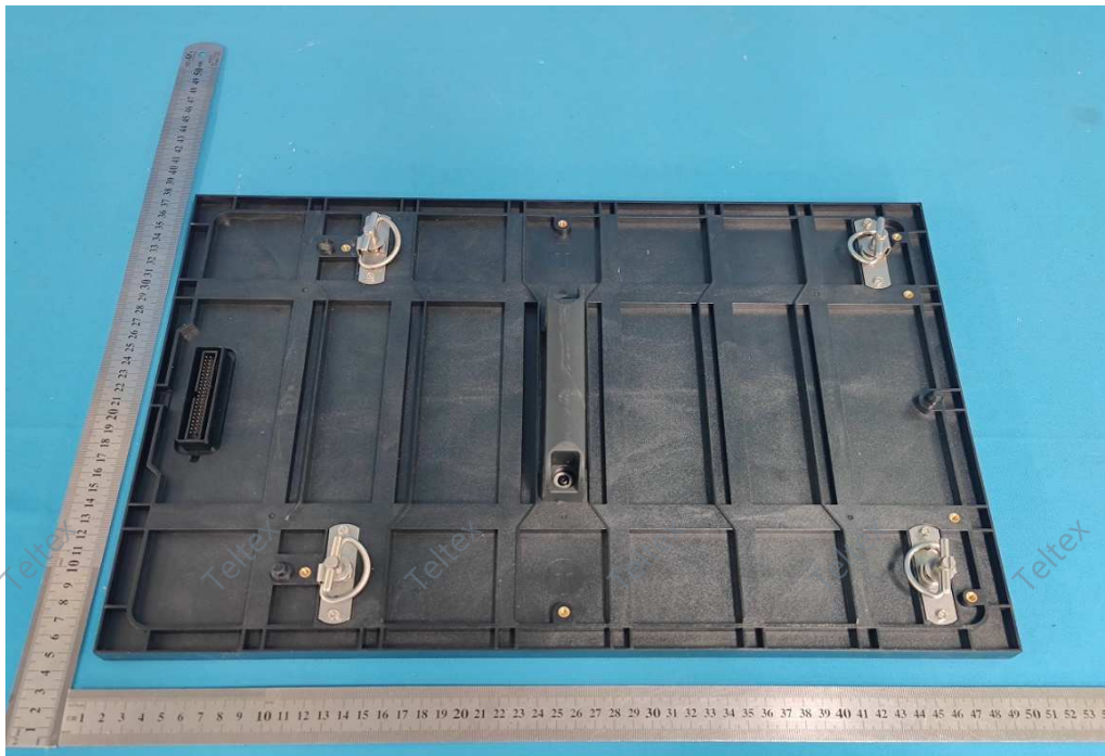
Photo 6 - LED Module view_2 Plastic bottom shell
