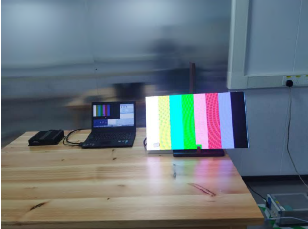
Photograph 3: Set-up for Conducted Emission from the AC mains power ports
