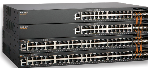
Figure 1: Up to 12 Ruckus ICX 7250 Switches can be stacked together using up to four full-duplex SFP+ 10 Gbps ports for a fully redundant backplane with 480 Gbps of aggregated stacking bandwidth.
